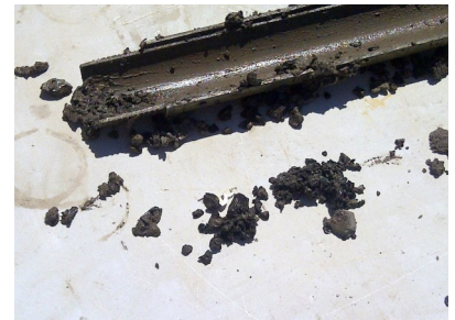
Fig. 2—Collecting soil samples from borehole
